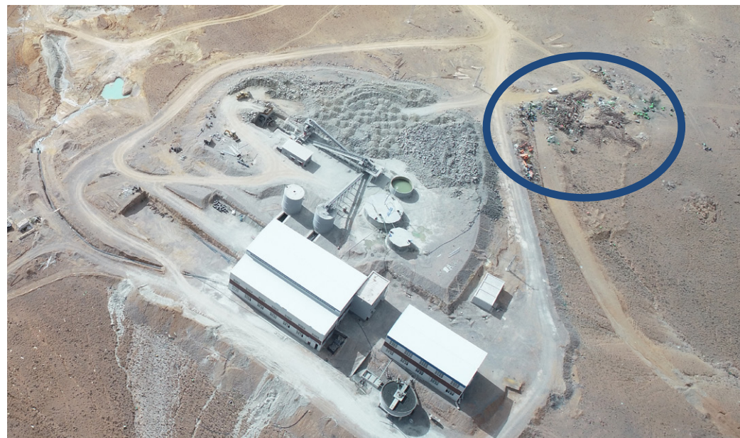
Metal scrap mixed with plastics, empty oil barrels, and anything else that can be found on a mine site. This site is located beside the flotation process plant, and from Google Earth satellite imagery it appears that the waste accumulation started with the construction of the flotation plant in 2018.
